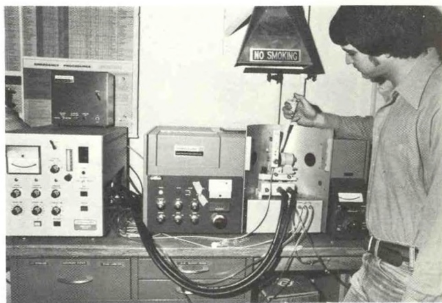
Technician using the atomic absorption spectrophotometer to analyze water samples in the chemistry laboratory. The graphite furnace added this past year upgrades the trace metal analysis capability.
