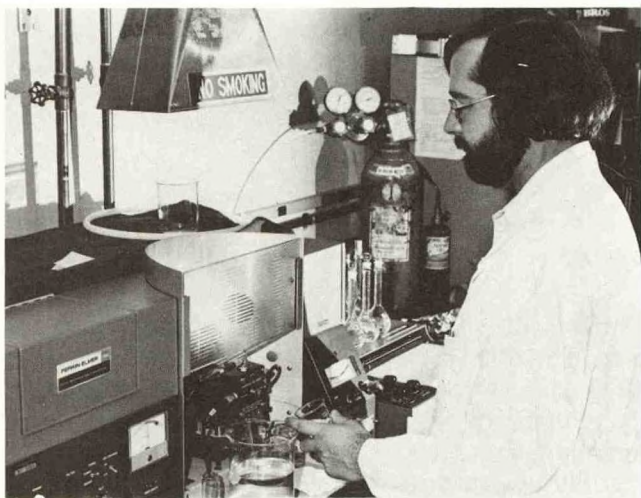
Scientist performing atomic absorption spectrophotometry for toxic trace metals. Other equipment in the chemistry laboratory includes an AutoAnalyzer.
