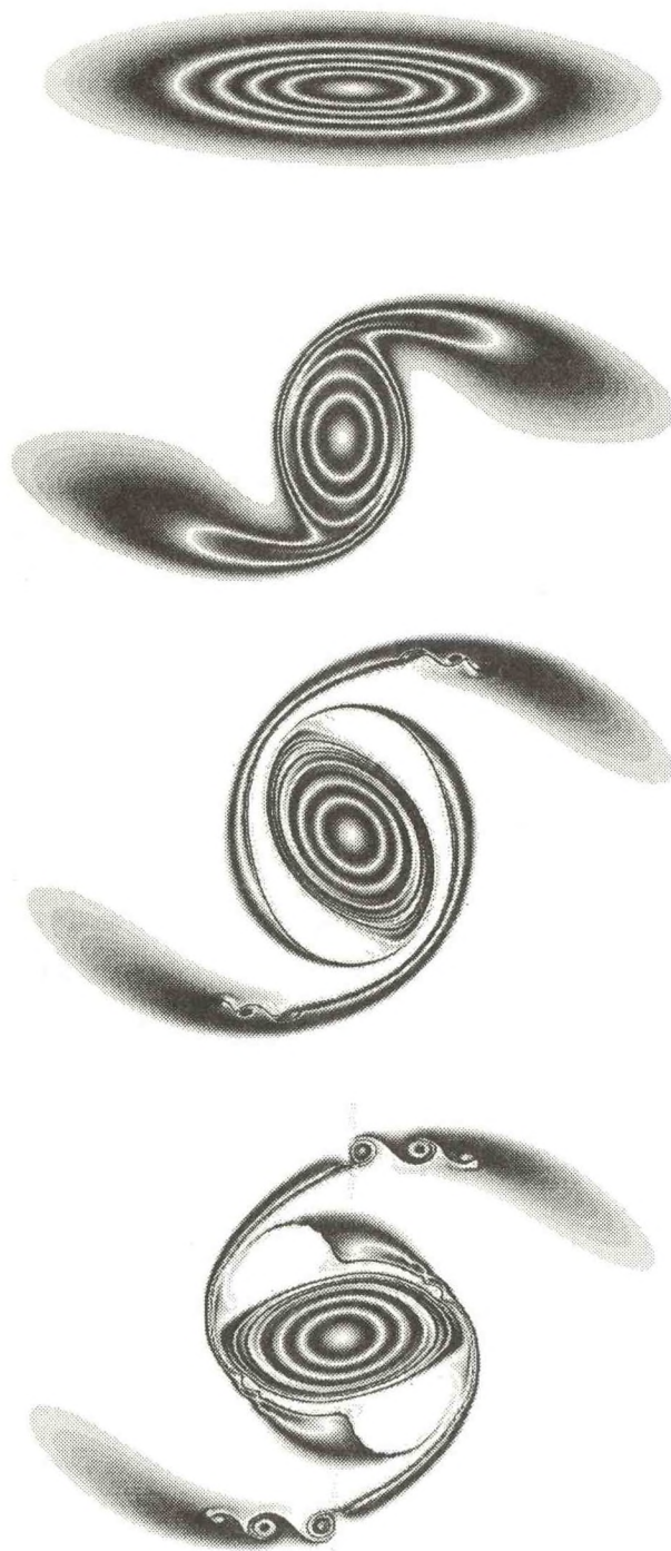
Fig. 1.10 An example of surface geostrophic dynamics. The flow is quasi-geostrophic in a semi-infinite domain over a flat surface, with uniform potential vorticity in the interior. The initial surface temperature distribution (upper panel) is \exp(-x^2 - 4y^2) , which is balanced by a surface cyclone. The remaining panels show how surface temperatures evolves in time.
