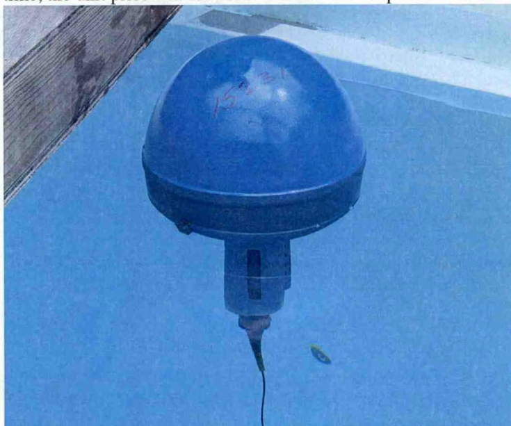
Figure 3. The SeaBird Microcats adapted to observe sea surface salinity (SSS) at the bottom of the SVP drifter float in the SIO test pool; 20 SVP-SSS test drifters have been deployed in the East China Sea to study the effects of the decreasing flow of the Yangtze on the ecology of South Korea.
