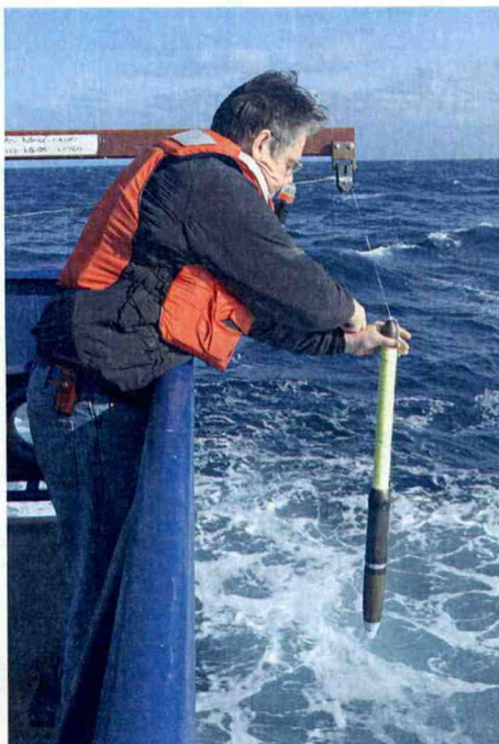
Figure 1. The UCTD being deployed from the R/V Revelle in April 2003.
