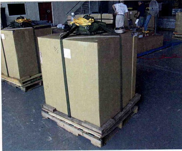
Figure 4. The JIMO/Minimet wind-sensing air-deployment container during tests at Keesler AFB in July 2003. A parachute is on top of the container and 2 Minimet drifters are inside the container. Upon deployment at sea, salt pills at the bottom of the straps dissolve in seawater in 20 minutes, releasing the parachute harness.
