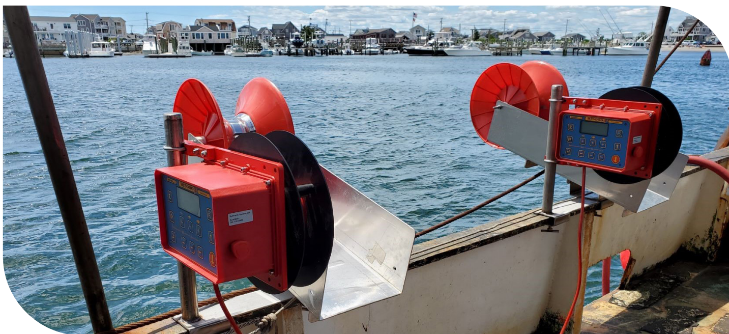
Automatic squid jigging machines set up on a Rhode Island-based trawl vessel. Credit: CFRF, Commercial Fisheries Research Foundation
