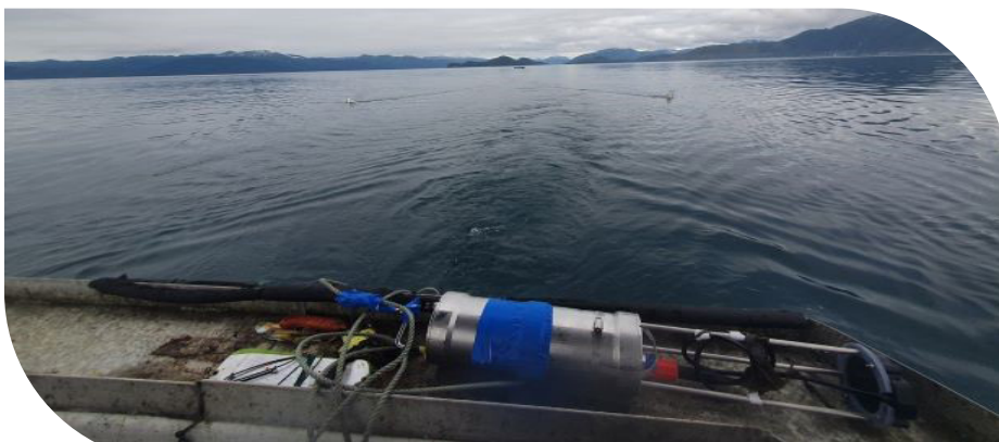
The fisheries pod ready to be deployed off the back of a commercial salmon troller in Southeast Alaska. Credit: Thomas Goetz
