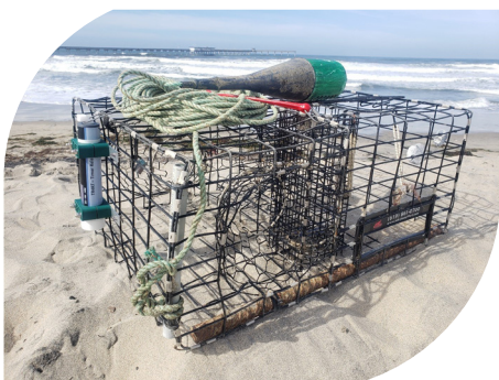
The timed release system developed by Coastal Monitoring Associates installed on a spiny lobster trap. Credit: Bart Chadwick.
