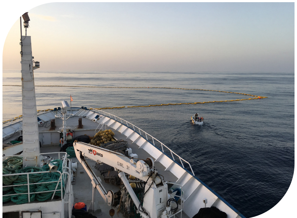
A small boat carrying scientists and scientific echosounder equipment from a large purse seine vessel to an enclosed tuna aggregation to take acoustic readings. Credit: Udane Martinez – AZTI.
