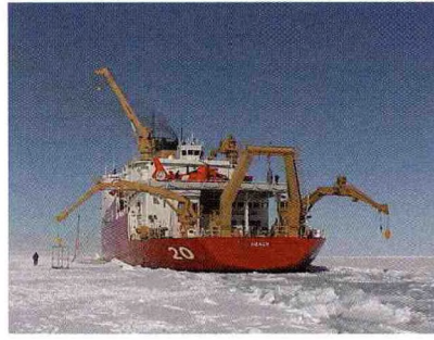
Figure 3-DOT-7. USCGC HEALY, the Coast Guard's new icebreaking research vessel, conducting ice trials.
