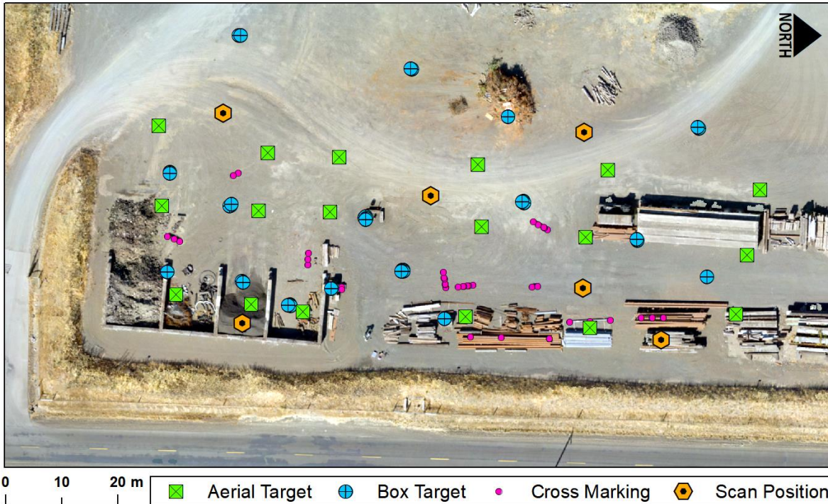
231 232 Figure 6: Location of the established aerial targets, cross markings, box targets, and scan positions
