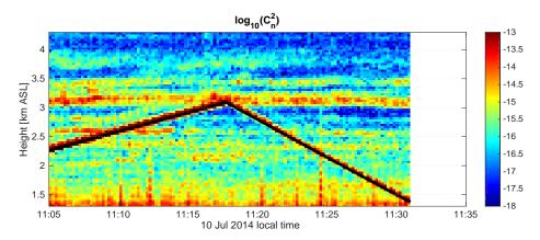
**Figure 5.** The black line represents the DataHawk altitude as a function of time plotted on top of the calibrated range-corrected received power for the morning flight (11:05–11:30). The DataHawk was dropped by a tethered balloon at an approximate altitude of 2.25 km. In this case, there is an ascent from its initial altitude to 3 km, followed by a descent over SOUSY down to 1.5 km.
