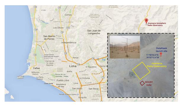
**Figure 1.** The Jicamarca Radio Observatory (JRO) is the experimental site for the observational campaign. JRO is located approximately 25 km from the city of Lima. The DataHawk launch site is on the JRO property 400 m from the main antenna (marked in yellow). The SOUSY radar is located next to the main antenna (marked in red). A picture of the SOUSY antenna elements is presented in the top left corner of the dash rectangle.
