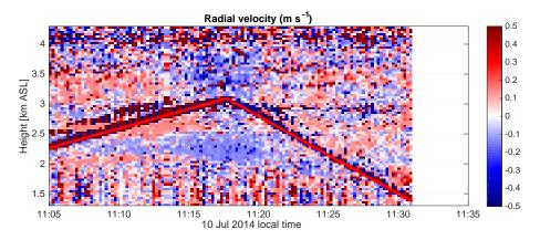
**Figure 6.** Corresponding radial velocity for the morning flight (same period as Fig. 5). The DataHawk trajectory is indicated by the red line. Vertical wind cannot be determined by the radar along the DH path due to strong returns from the DH vehicle.
