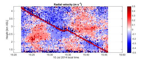
Figure 12. Similar to Fig. 6 but for the afternoon flight. Estimates of the vertical wind cannot be estimated from radar returns along the DataHawk path due to its high reflectivity.
