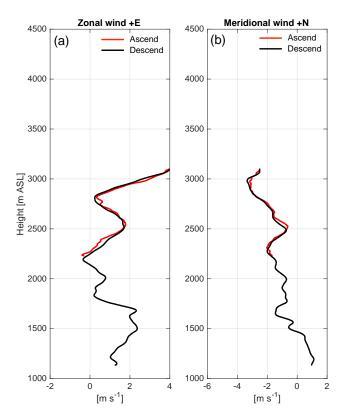
**Figure 7.** Horizontal winds obtained from the DataHawk for the morning flight. (a) Zonal wind. (b) Meridional wind. The red line indicates the ascent portion of the flight, while the black line indicates the descent portion of the flight.
