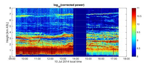
**Figure 3.** SOUSY daytime calibrated range-corrected received power for 10 July 2014 shows distinct turbulent layers from 500 m up to 7 km. The dropout of data between 14:00 and 15:00 was due to upgrades in the radar system that allowed for discrimination of echo returns bellow 1 km. DataHawk flights over the radar were easily detected as an increase of the radar returns between 11:05 and 11:30 and between 15:21 and 15:46.
