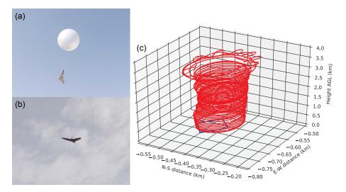
**Figure 2.** (a) Balloon lifting the DataHawk for the afternoon data set on 10 July 2014. (b) DataHawk flying towards the landing site for the same data set at an approximate altitude of 50 m. (c) Helical trajectory of the DataHawk descending from approximately 3.75 km to 500 m over the SOUSY radar (indicated in blue).
