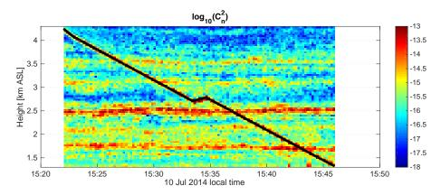
**Figure 11.** Similar to Fig. 5 but during the afternoon flight (15:21–15:46). In this case, the DataHawk was dropped by a "free" balloon at an altitude of approximately 8 km. However, due to the strong winds, the DataHawk was advected 4 km from the SOUSY radar, which caused a 3 km drop during the time it took to regain its position over the radar.
