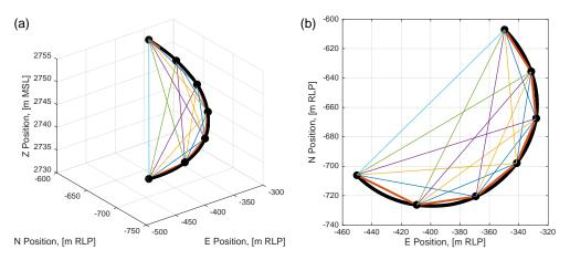
Figure 8. Illustration of a method for evaluating  $C_n^2$  (adapted from Wainwright et al., 2015; Bonin et al., 2015) for a helical trajectory. The different distances  $\delta_E$  are represented by the lines with different colors. The measured points are indicated by the black dots. The smallest distance used in the DH direct method is indicated by the thick red line. (a) 3-D view of the trajectory for a portion that covers at least one half circle. (b) Top view of the trajectory.
