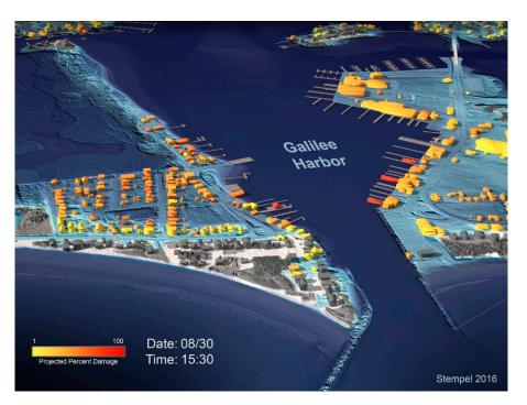
**Figure 1.** Excerpt from time incremented 3D hazard visualization series of Galilee Harbor, South Kingstown, RI, USA, depicting the progressive impacts (%structural value) of Hurricane Carol (1954) at current sea level on present build-out. The impact modeling system used to drive this visualization is currently adapted to real-time deployment for use by emergency managers. Image: Authors.
