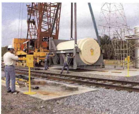
Figure 3-NRC-1. NRC regulates the storage of spent fuel at nuclear plants. The photo shows a fuel cask being maneuvered in a cradle at the Hatch plant in Georgia.
