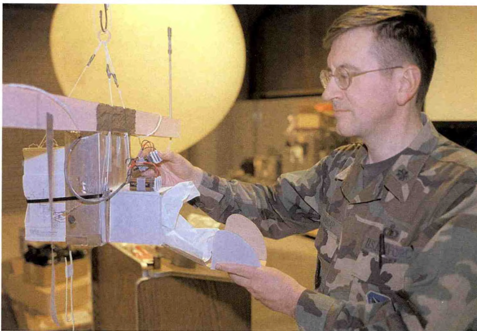
Figure 3-DOD-4. An AF weather officer prepares a balloon for measuring atmospheric turbulence conditions as part of the airborne laser program. (US Air Force photo by Staff Sgt. Timothy Cook)
