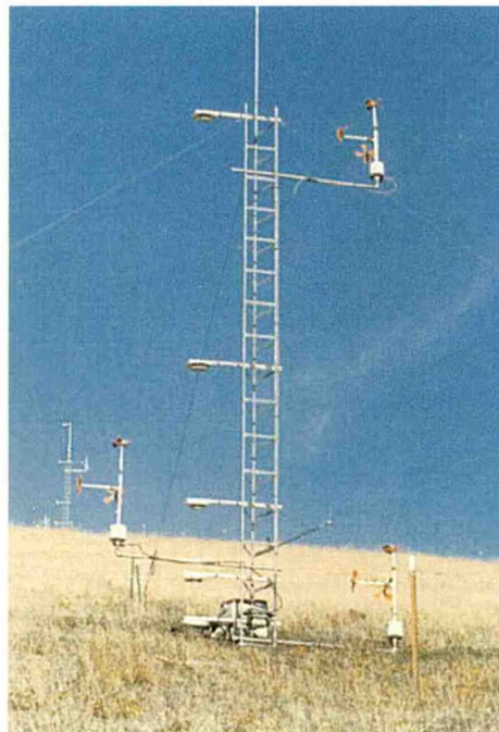
Figure 3-DOE-2. Meteorological towers record temperature and wind direction and speed at various levels. at 2m, precipitation, and global solar radiation, eleven provide barometric pressure. The other three towers range from 46 to 76m in height and are instrumented at multiple levels. The sensors at all stations are scanned every second and averaged or totaled over five minutes.
