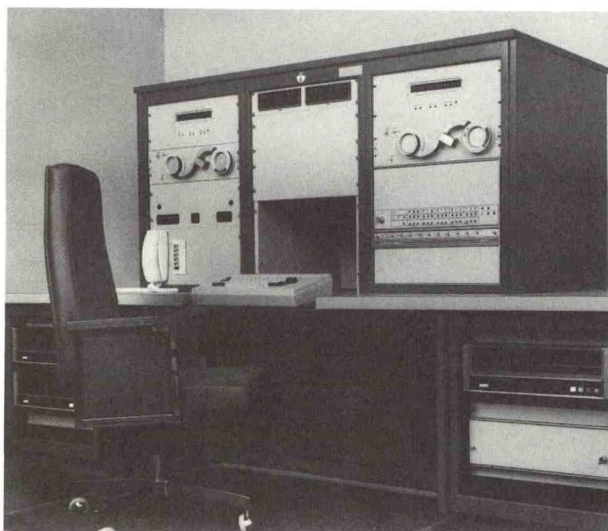
AFOS Supervisory Console containing the mini-computer, disc storage, modems, and data archival tape units.
