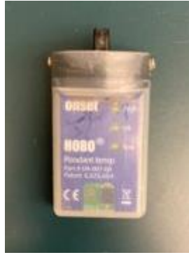
Figure 12. Thermometer used to monitor water temperature (in degrees Centigrade) in the tank
