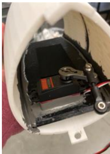
Inside shelf and servo attached to the interior of the body.
