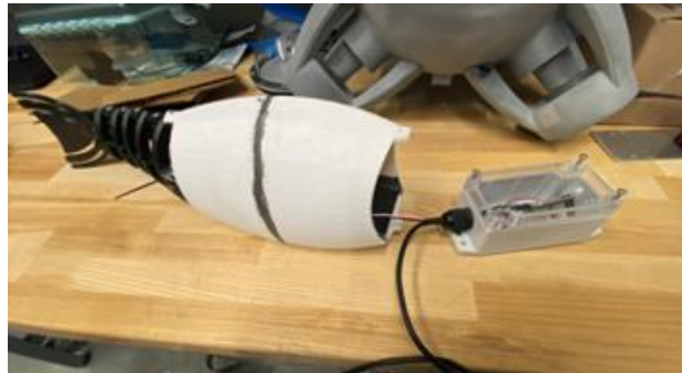
Modularity of safety box as it is taken out of the body.
