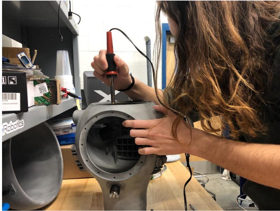
Threaded Heat Inserts Installation into the Hull
