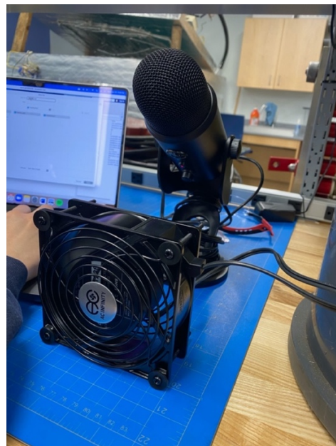
Figure 7: Fan and microphone experimental setup.
