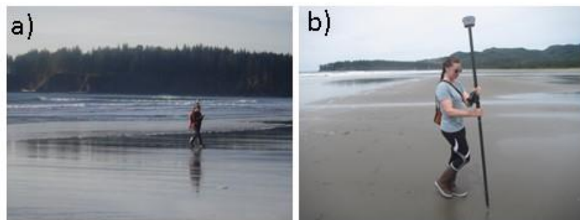
Figure 3. Surveyors walking cross-shore oriented transects on Hobuck Beach with GNSS systems mounted on an a) backpack or b) 2.0-m rover pole
