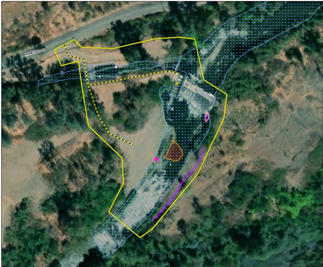
Figure 1. Aerial view of the Project area. Yellow = study area, light pink = permanent impacts to Waters of the U.S., purple = permanent RSP above the OHWM, and orange = temporary impacts to Waters of the U.S. from a temporary gravel pad. The dark pink star represents an existing fyke pipe outfall.
