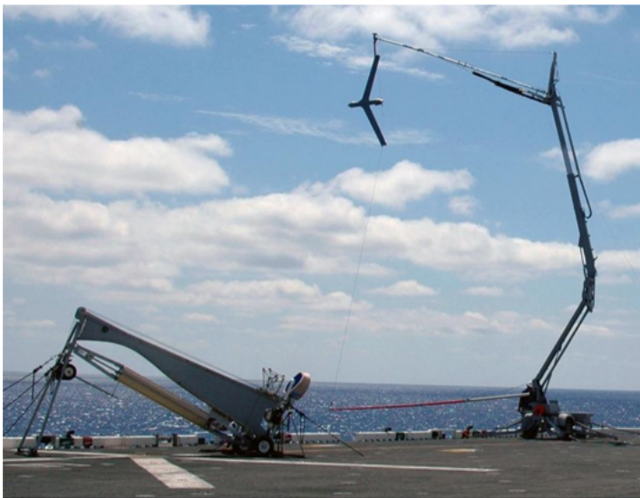
Figure 4. The Boeing Insitu “ScanEagle” UAS is a LALE platform that requires a portable, catapult-assisted launch system (left) for take-off and a retractor system known as “Skyhook” (right) for landing
