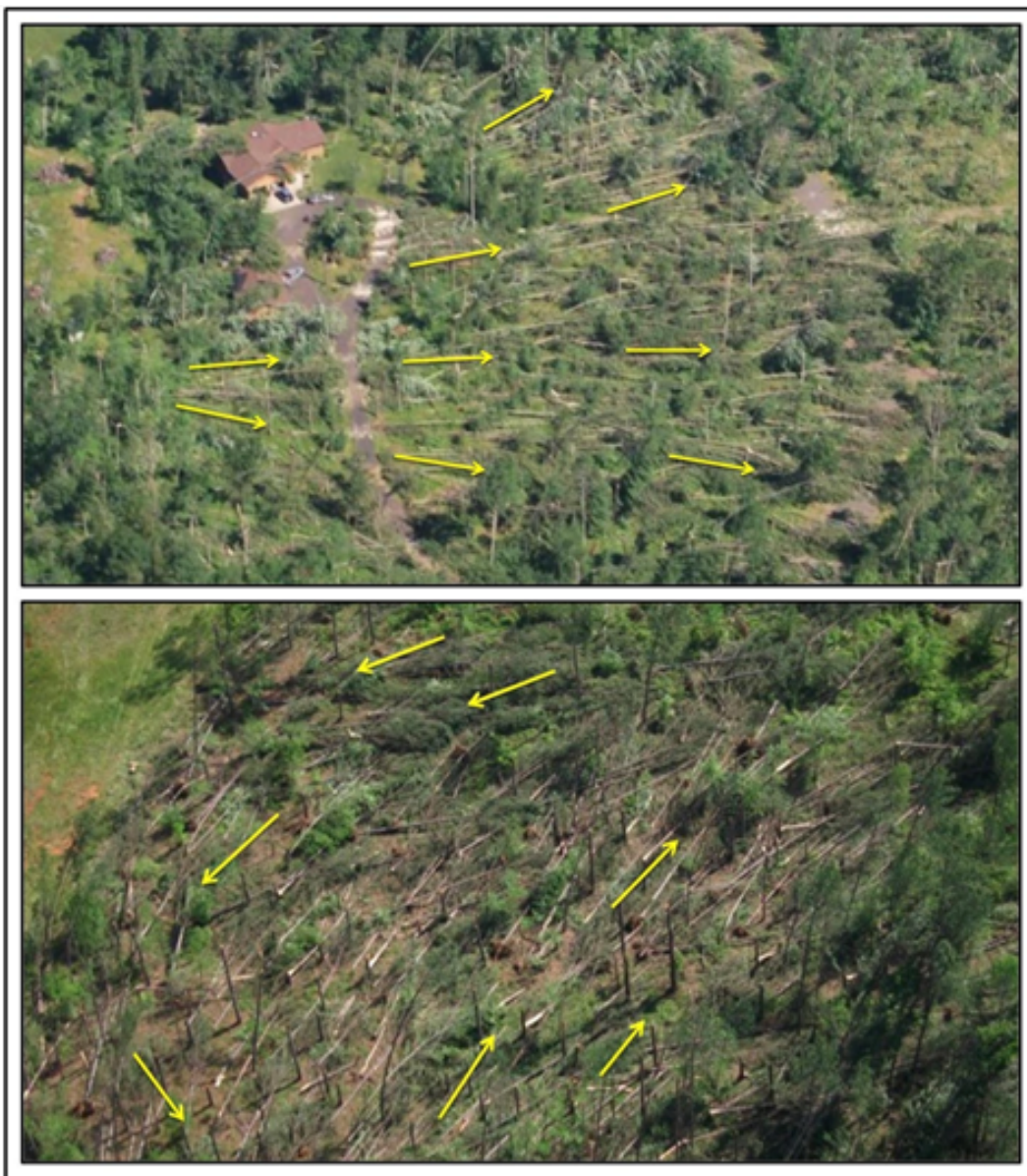
Figure 5. An aerial perspective can aid NWS damage surveyors in distinguishing straight-line wind damage (top) from tornado damage (bottom) by looking for fanned-out (top) or convergent (bottom) tree-fall patterns. Images provided, courtesy of NWS forecast offices in Duluth, Minnesota, and Huntsville, Alabama, respectively.
