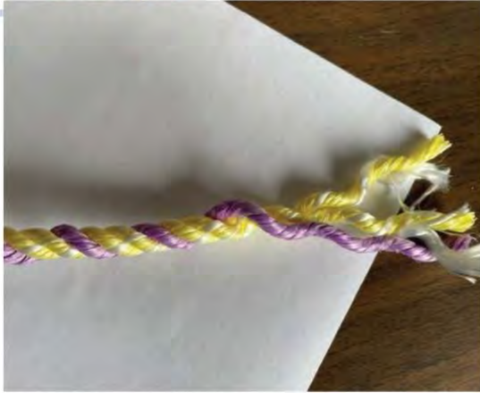
Dyed yellow Hydropro (neutral Buoyancy) and dyed purple Polysteel (floating) strands twisted together
