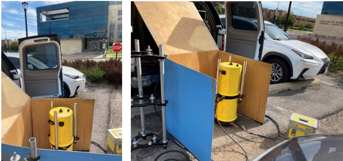
Figures 2 (a) and (b). A10 site looking East and Northeast with blue wind shelter and gradient tripod depicted.
