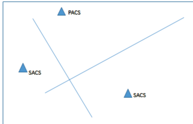
Figure 26. Simplified airport geodetic control schematic showing PACS/SACS (triangles)
