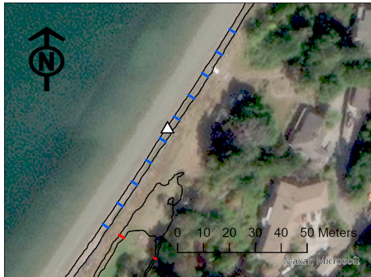
Figure 4. Visual verification of transects. In this example of an accretion shoretype, the random point is marked with a triangle, transects are arrayed at 10m intervals, five to either side. Blue transects on the seaward beach face were retained while red transects in the backshore were discarded.
