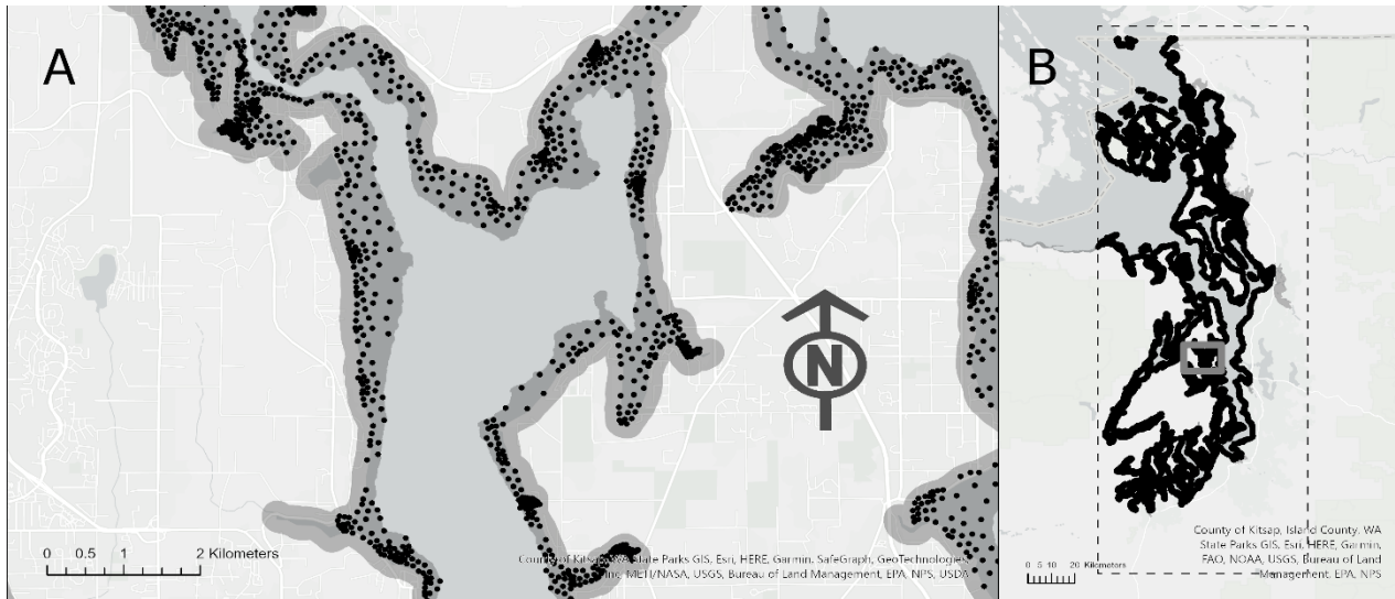
Figure 2. TCARI point distribution. 82,918 well distributed points provide a continuous estimate of HAT elevation within a nearshore zone. These points were a sub-set of a continuous grid developed by NOAA CO-OPS. Figure 2A shows the typical density of points within the nearshore zone. Figure 2B shows the position of Figure 2A, as well as the extent of the CoNED Model.
