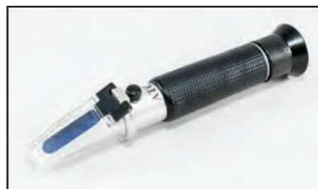
A refractometer is used to measure salinity.
