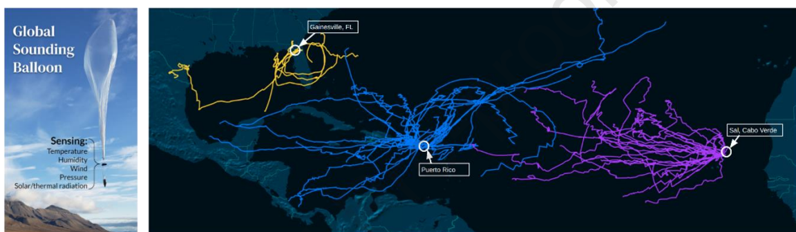
Figure 15: Fall 2022 Global Sounding Balloon Atlantic Flight Map — Trajectories of 85 Global Sounding Balloons launched from 3 sites over Sept-Oct 2022, showing the wide geographical reach possible with altitude-controlled long-endurance balloons.
