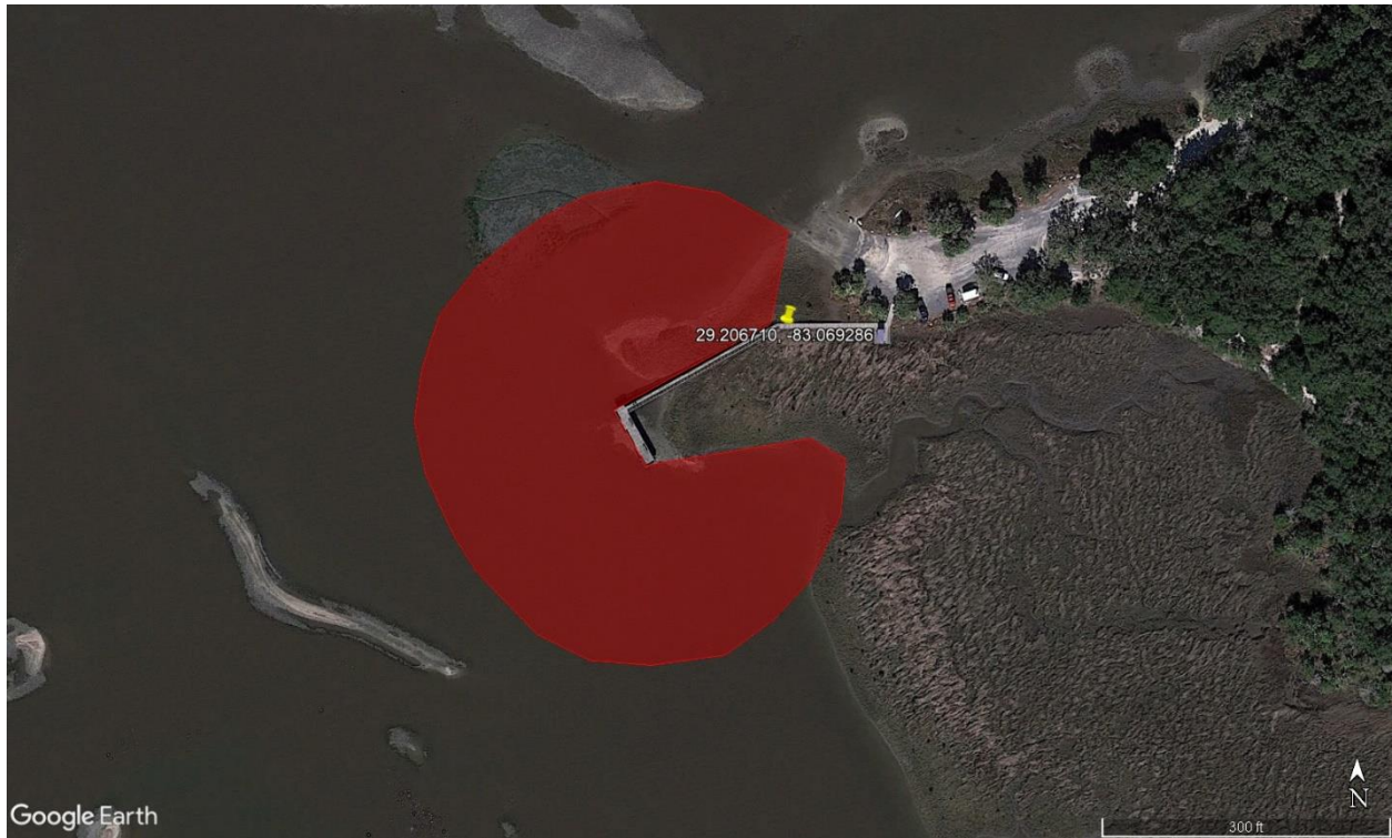
Figure 3. The extent of the action area as defined by the largest radius of effects on ESA-listed species based on the proposed installation of 9-in-diameter wood piles by vibratory hammer.
