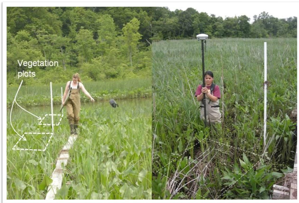
Figure 7-14. RTK GNSS within wetland vegetation plots. Note that only one corner of each plot is marked with the PVC cap; consistent field procedures need to be followed to approach sites and take positions at each corner.
