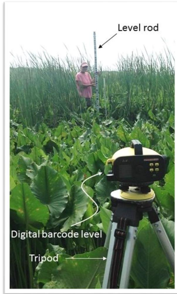
Figure 7-5. Leveling to a corner of a vegetation plot.
