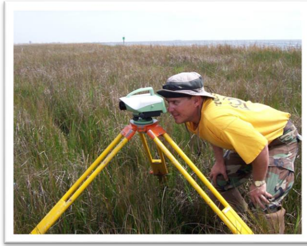
Figure 6-20. Leveling in the wetland: note splayed legs of tripod between 45° and 60° to enhance stability.
