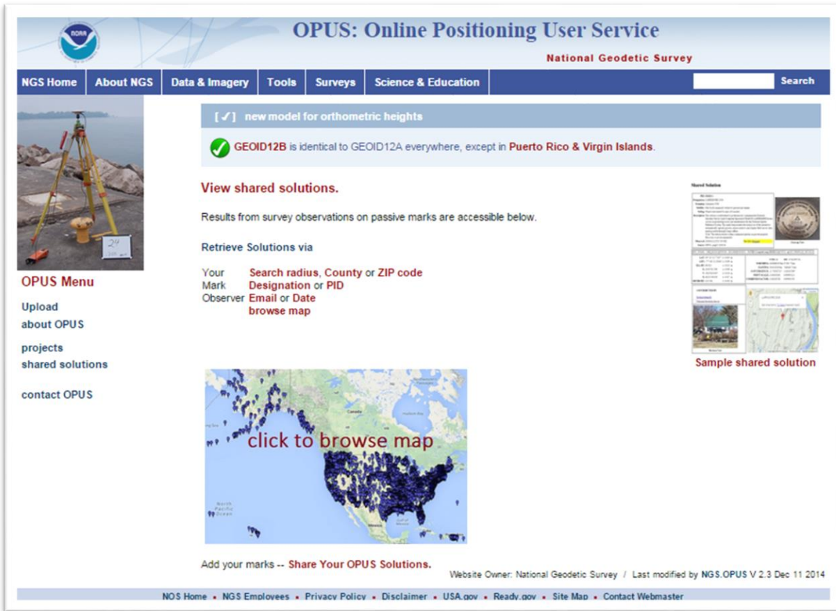
Figure 3-12. Screen capture showing OPUS “Shared Solutions” retrieval options and solution formats. Options include radial search, or search by county, zip code, as well as a map-based browser.
