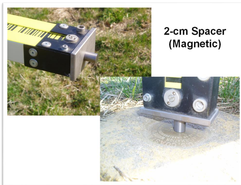
Figure 6-13. Matching (calibrated) 2-cm magnetic plugs used to place rod on vertical point of reference (VPR) where VPR is recessed, and calibrated end of rod cannot make direct contact. Both plugs must be used in the same setup (both backsight and foresight).
