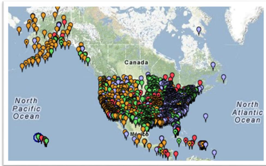
Figure 2-4. National CORS Network. The different colored marks refer to the different frequencies at which the GPS data are being collected and processed by NOAA.
