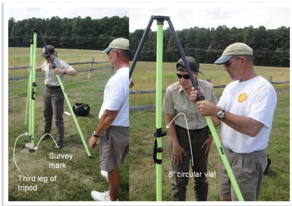
Figure 6-28. Plumbing a 2 m, fixed-height GNSS survey tripod. Left panel shows how to grasp the leg release levers. Note that the third leg is not deployed until the tripod is plumb. Right panel shows the two-handed technique for fine-tuning the adjustment.
