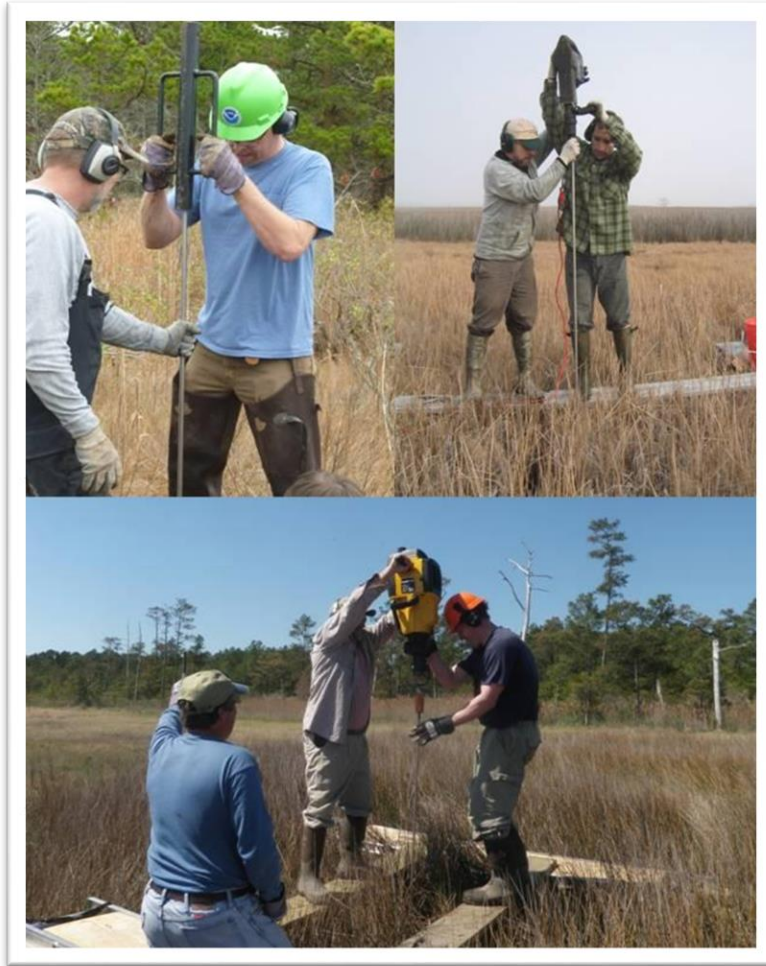
Figure 5-9. Three techniques for setting deep rod marks (or deep rod SET marks). These include using a hand-held pile driver (top left), a lightweight electric demolition hammer (top right), or a self-contained gasoline powered jackhammer (bottom).
