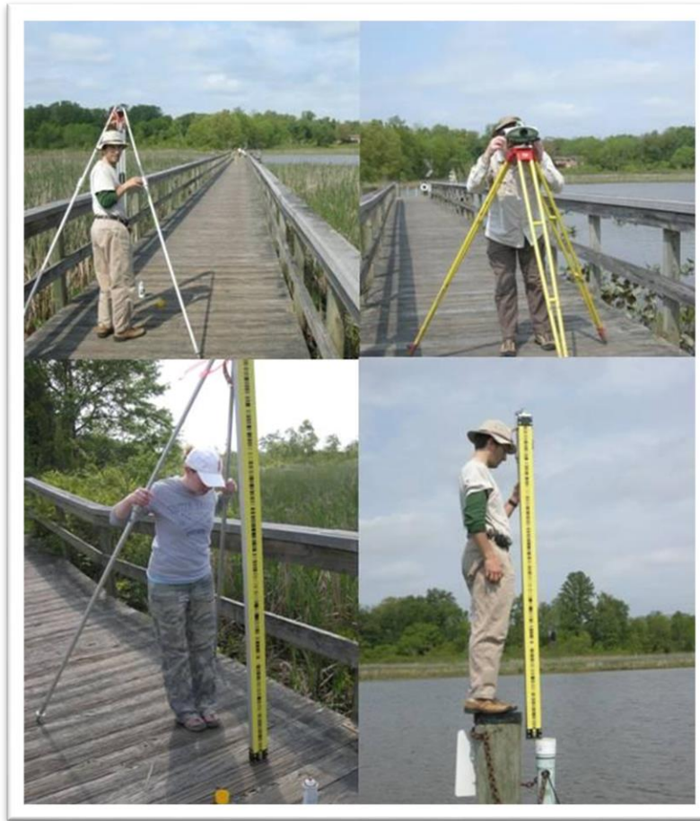
Figure 7-1. Digital barcode leveling from local vertical control network to the protective well of the water level sensor.
