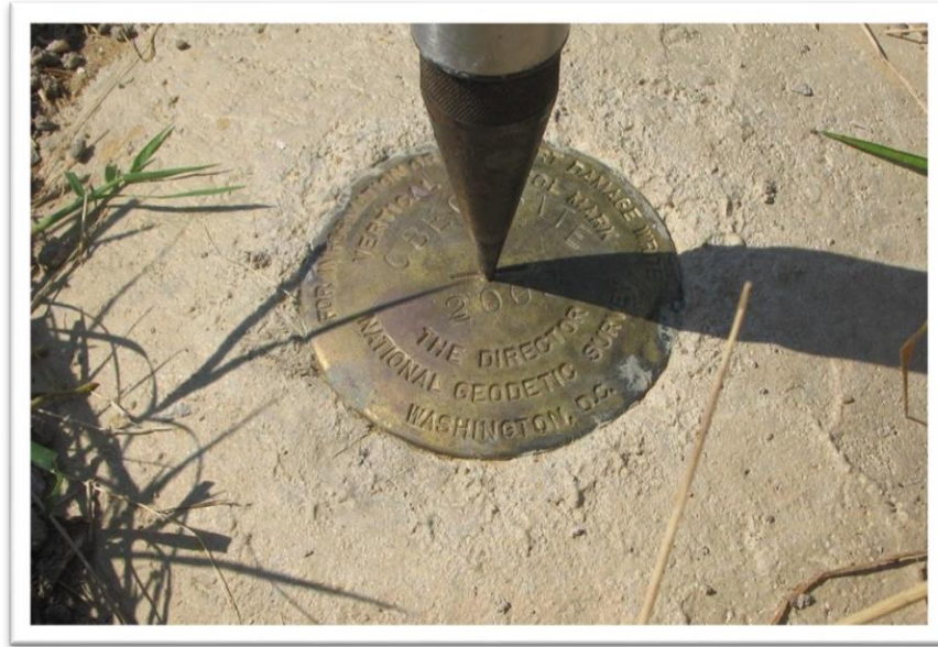
Figure 6-27. The survey point of a tripod is placed on the vertical point of reference of a typical metal survey disk.
