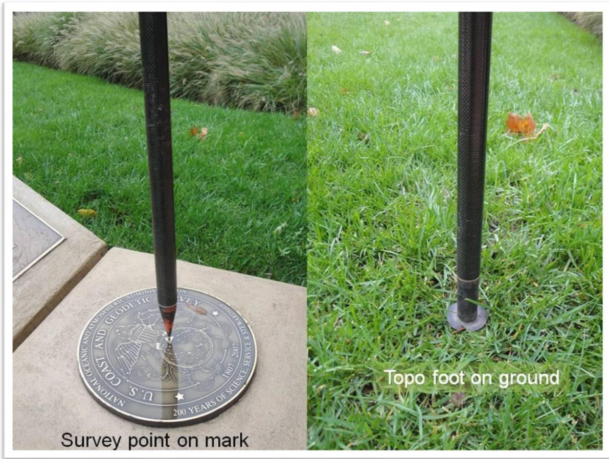
Figure 7-10. Close-up of two different kinds of rover tips. Left panel: survey point on mark; right panel: “topo foot” on ground. The base of the topo foot is approximately 2.5 inches in diameter.
