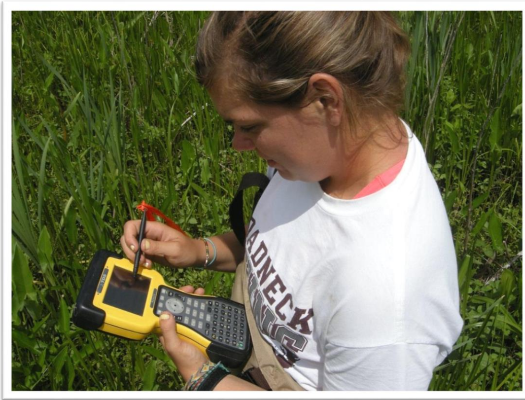
Figure 6-34. Hand-held data logger used to set up the job file and communicate with late model GNSS units.
