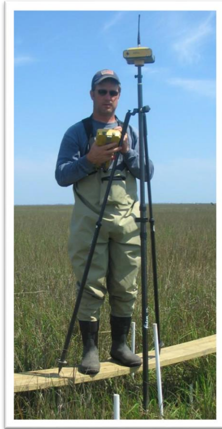
Figure 7-12. RTK on a SET foundation in the wetland. Note: that the RTK rover brace poles can rest on a wooden platform for stability.
