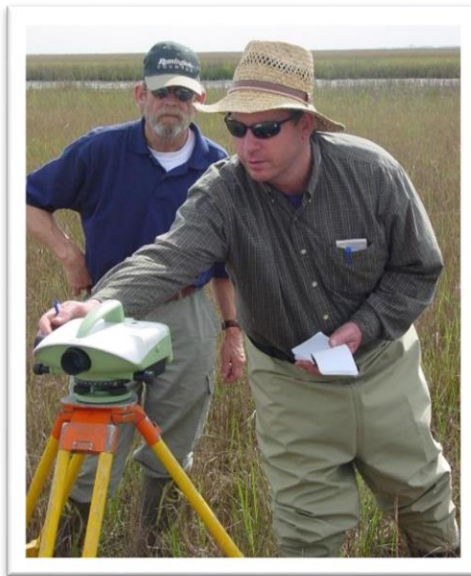
Figure 6-21. Leveling in the wetland: Operator(s) standing away from tripod, while activating electronic measurement.
