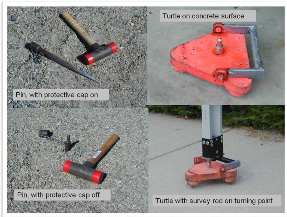
Figure 6-17. Pins and turtles used as turning points during a leveling section.
