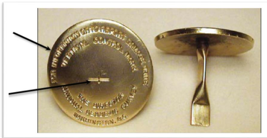
Figure 5-2. Survey marker that is used atop a concrete post mark. Note that the mark is slightly domed (which helps for leveling), but also has a small survey mark punched at the top, to facilitate GNSS-derived positions.
