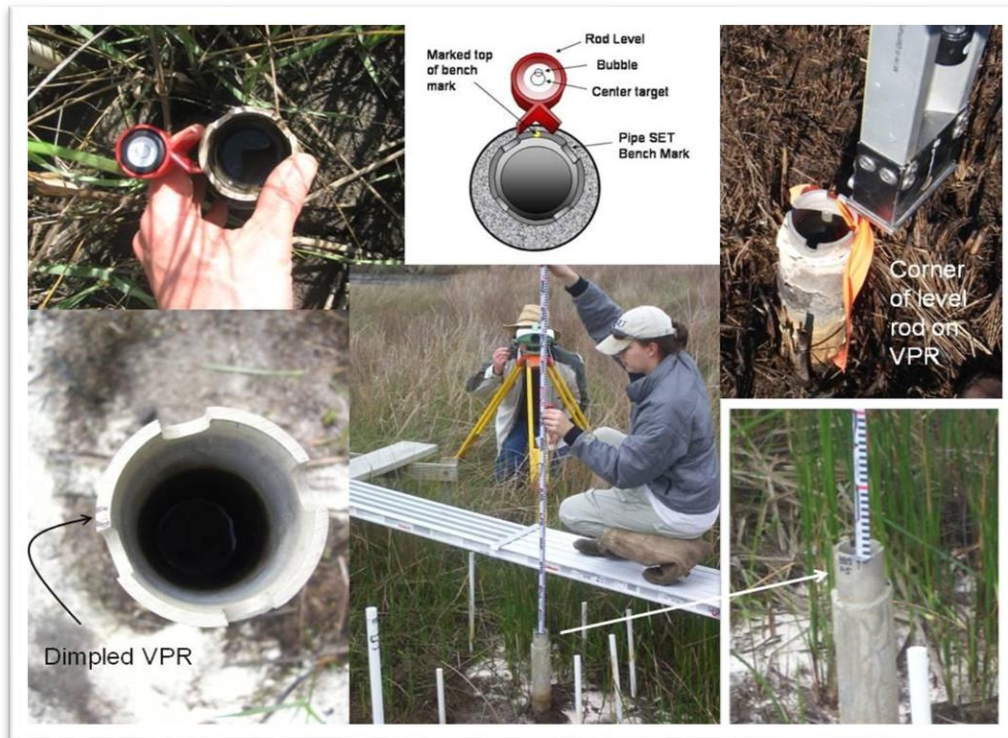
Figure 7-3. Procedures for finding and leveling to vertical point of reference of a first generation SET foundation.
