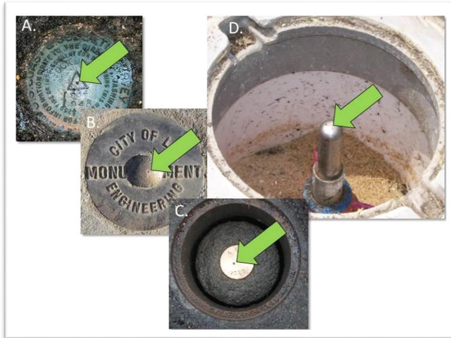
Figure 6-12. Examples showing different types of survey monuments and the location of the vertical point of reference (green arrows). A: typical domed brass disk; B: leveling disk with raised center; C: Brass cap on metal rod encased in pipe; D: deep rod mark with domed datum point.
