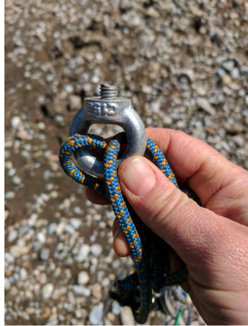
Figure S5: Rock anchors at an antenna in the upper Carmel River, California. The block anchors with eye bolts held for part of a season, but then broke at the bolt during a high flow event.
