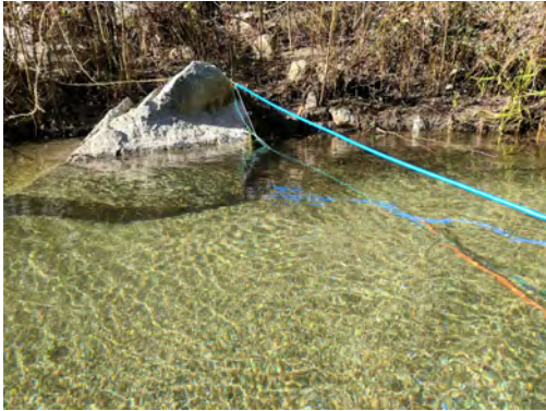
Figure S5: Rock anchors at an antenna in the upper Carmel River, California. The block anchors with eye bolts held for part of a season, but then broke at the bolt during a high flow event.
