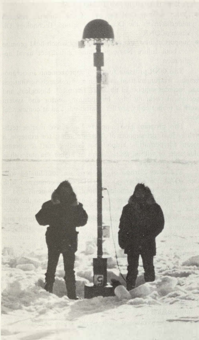
Figure 35.—AIDJEX ice buoy.
