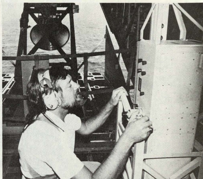
Figure 30.—NOAA airborne laser profileometer for measuring wave heights, used during WISEX (Winter Storm Experiment).
