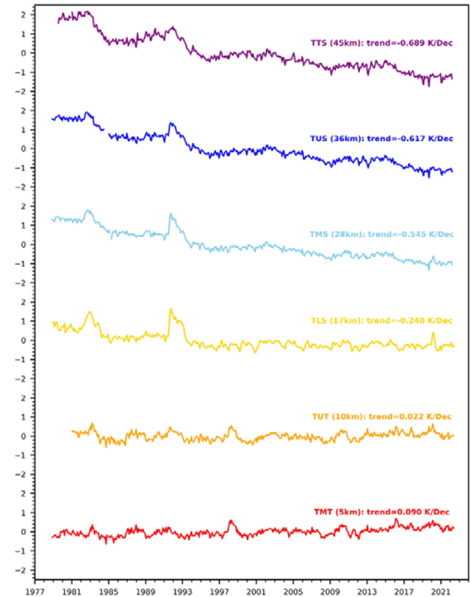
Figure 13. Deseasonalized monthly global mean temperature anomaly time series and trends for the mid-troposphere (TMT), upper-troposphere (TUT), lower-stratosphere (TLS), mid-stratosphere (TMS), upper-stratosphere (TUS), and top-stratosphere (TTS). The heights in the brackets above each time series represent the peak levels of weighting functions for each instrument channel measuring the temperature index time series. Trends were calculated for the period from January 1979 to June 2021.
