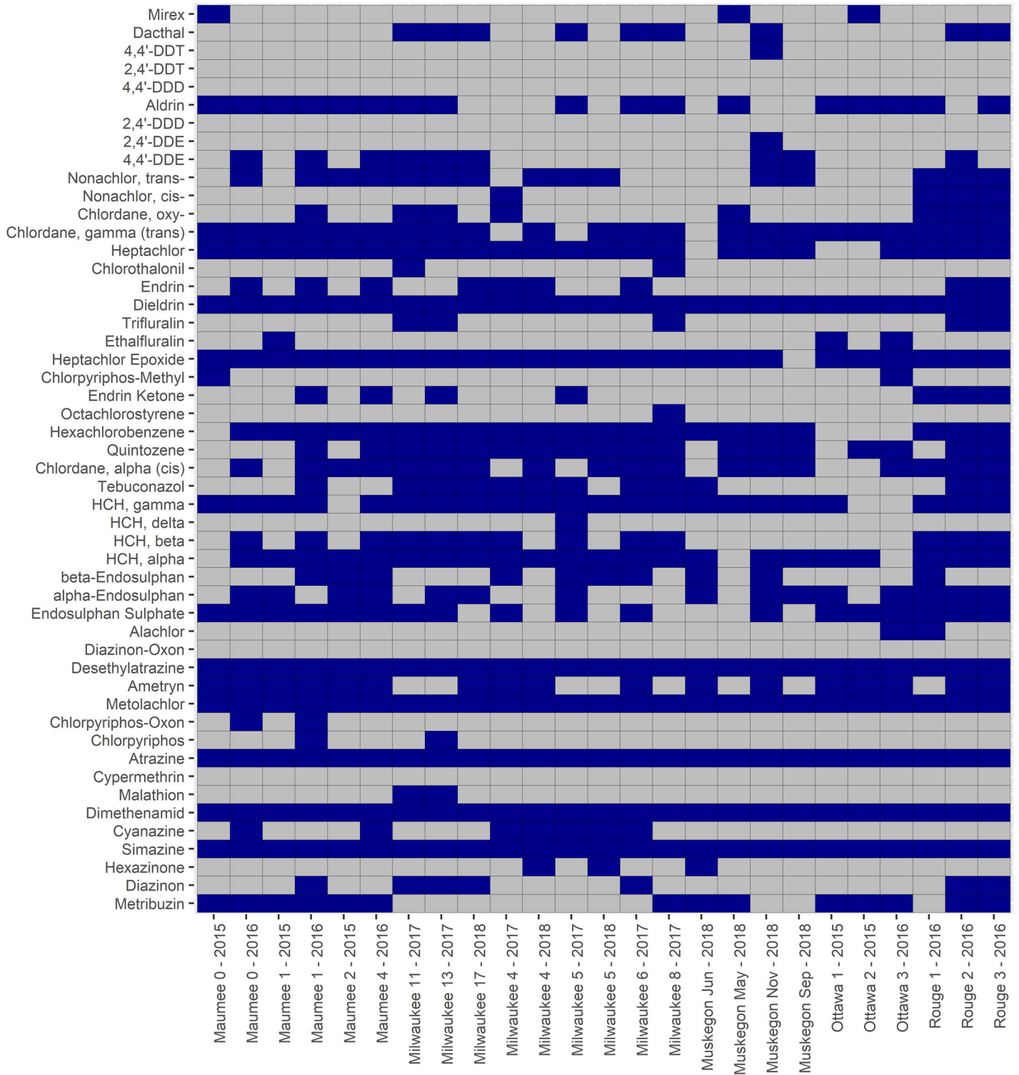
Figure 7. Heatmap of all pesticides detected in POCIS across all deployments. Compounds are organized by LogKow value, with values increasing from bottom to top. Dark blue cells (█) indicate presence of a given compound in POCIS, whereas grey cells (■) indicate absence of a compound.
