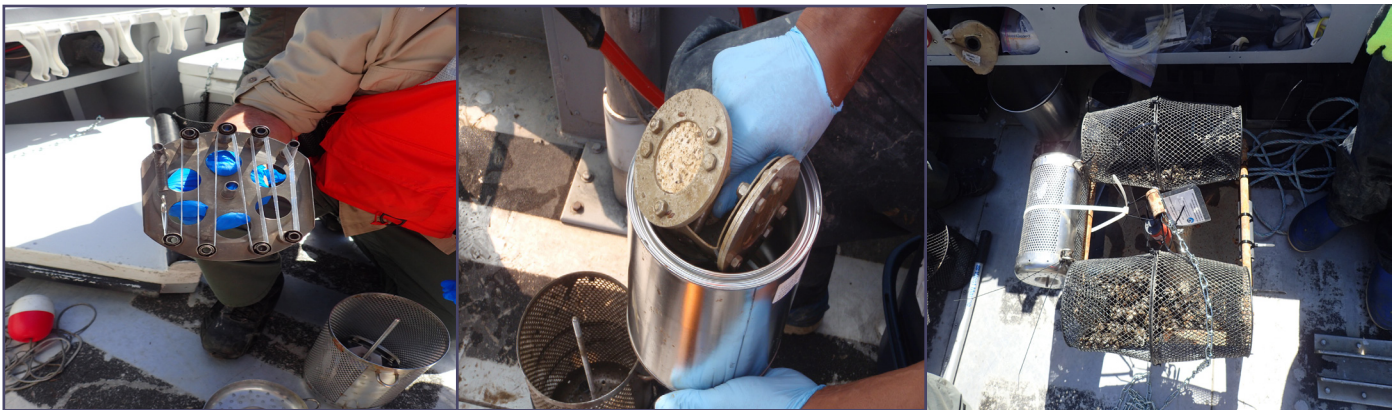
Figure 2. Example of the SPMD passive sampler (left), POCIS passive sampler (middle), and caged mussels (right). SPMD and mussels are shown pre-deployment, with the POCIS shown post-deployment.
