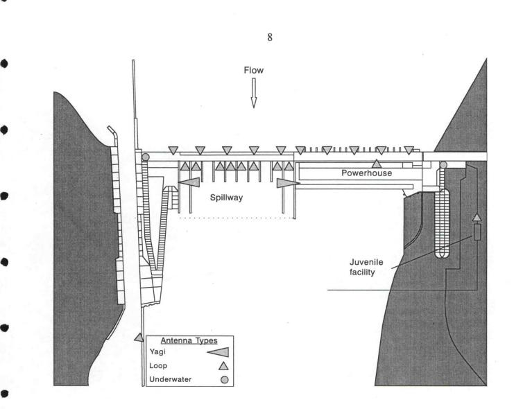
Figure 2. Ice Harbor Dam depicting locations of telemetry receivers and types of antennas (study area entrance and exit lines are not shown). Symbol direction indicates the primary detection area of a given antenna.
