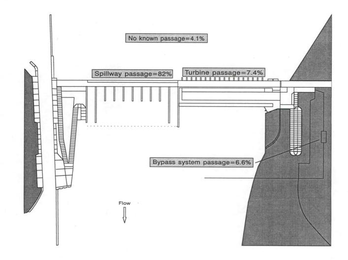
Figure 5. Passage distribution for radio-tagged hatchery-reared subyearling chinook salmon at Ice Harbor Dam, 1997. (Note: Radio-tagged fish with records on the entry and exit lines but with no record of passage at the dam were assigned turbine passage).
