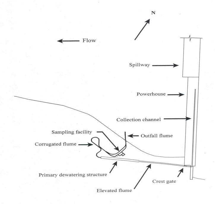
Figure 1. Overhead view of John Day Dam showing major components of the juvenile bypass system.
