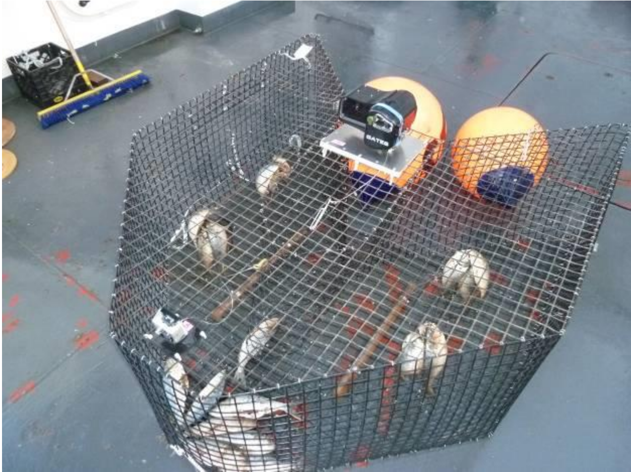
Figure 1. Chevron trap with video cameras attached over the nose and mouth positions.
