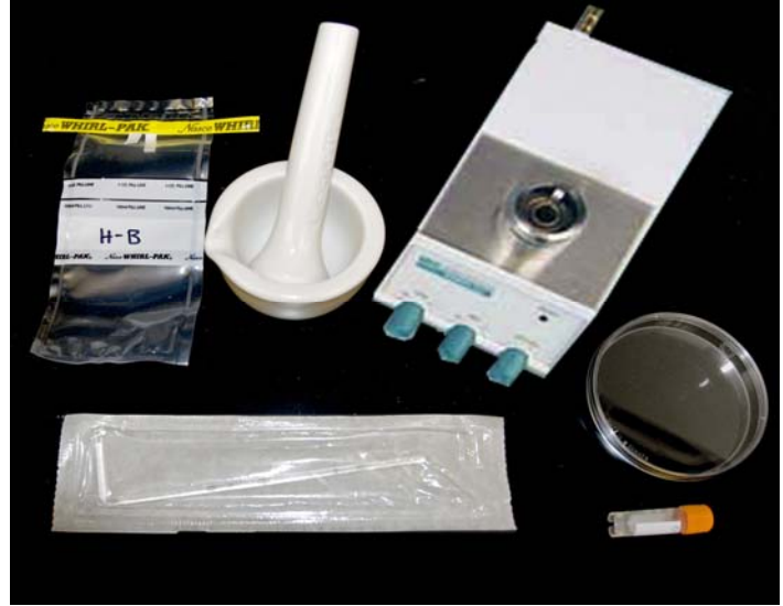
Figure 4.7.2.4 Equipment used in processing tissue samples for microbiology. These include a mortar and pestle for grinding fresh tissue, device to flame sterilize spreading rods, agar plate for culturing bacteria and cryovial for freezing ground tissue sample.
