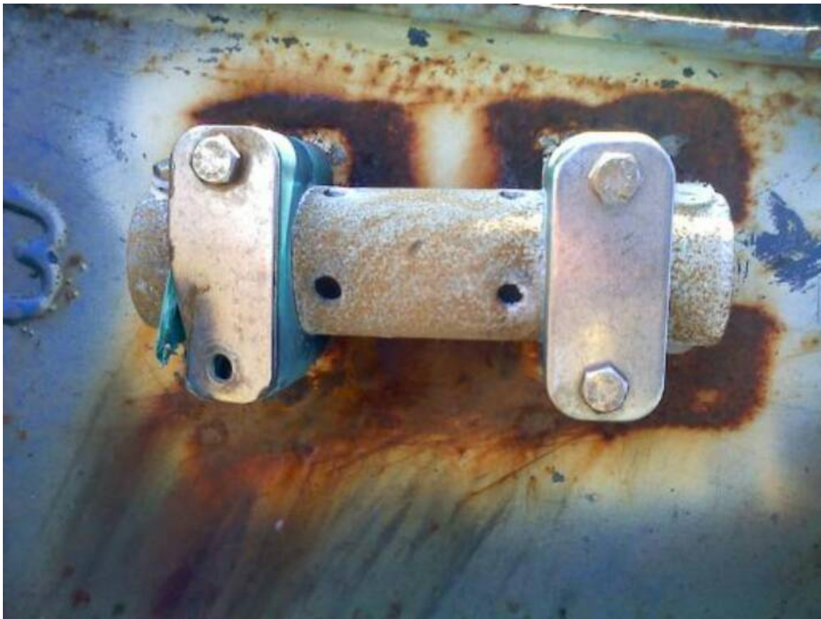
Figure 8. Condition of the tow time data logger housing after 3 yr, 4 mo, and 11 da.
