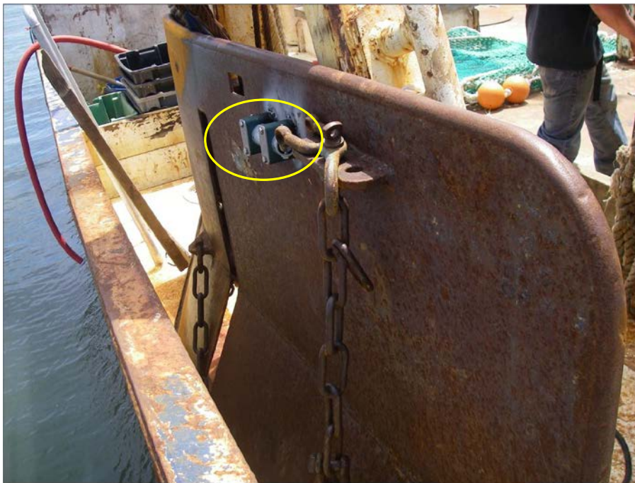
Figure 7. One common tow time data logger mounting location is on the outside of the trawl door near an eye and shackle.
