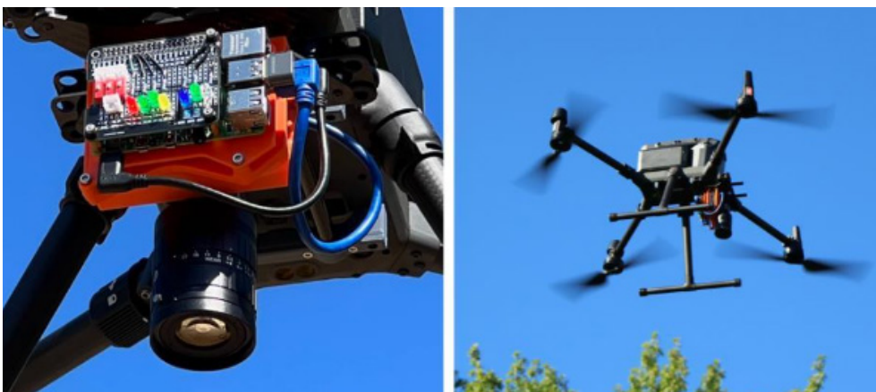
Figure 11: Blackfly-S polarimetric camera integrated on DJI Matrice 300. Credit: Oregon Statue University.
