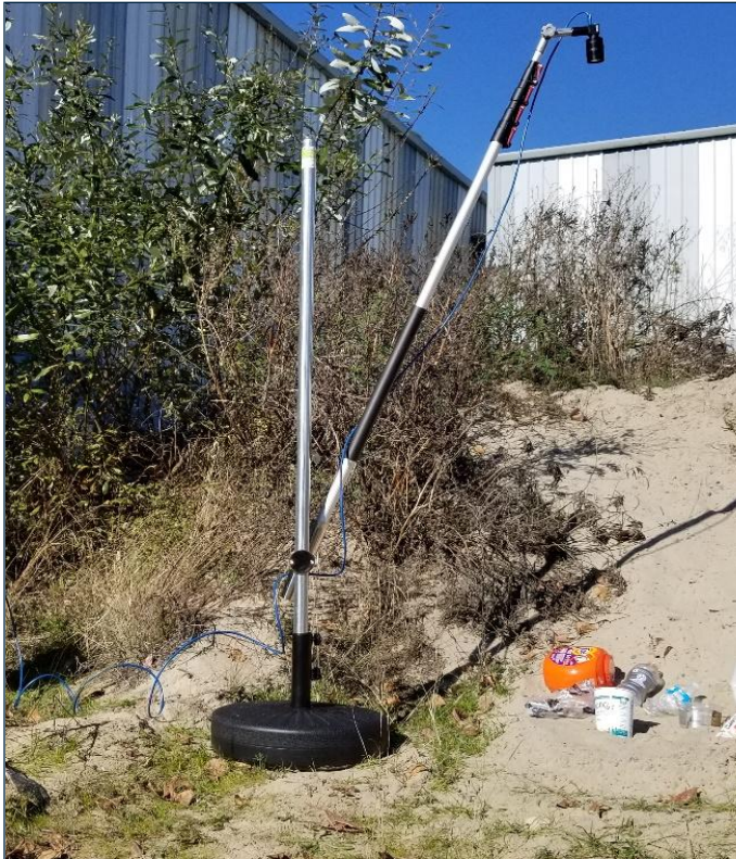
Figure 7: Pole-mounted PI camera set up at Hinsdale Wave Lab. Here the FLIR Blackfly S USB3 PI camera is operated from a pole in a weighted stand and connected to a field laptop (out of the photo, to the left). Credit: Oregon State University.
