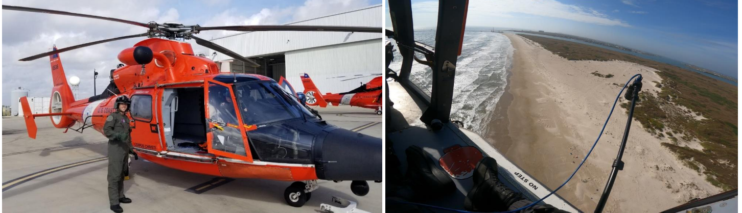
Figure 10: Tests of PI camera on USCG MH65 Echo helicopter to simulate UAS polarimetric imagery acquisition. Credit: NOAA NCCOS.
