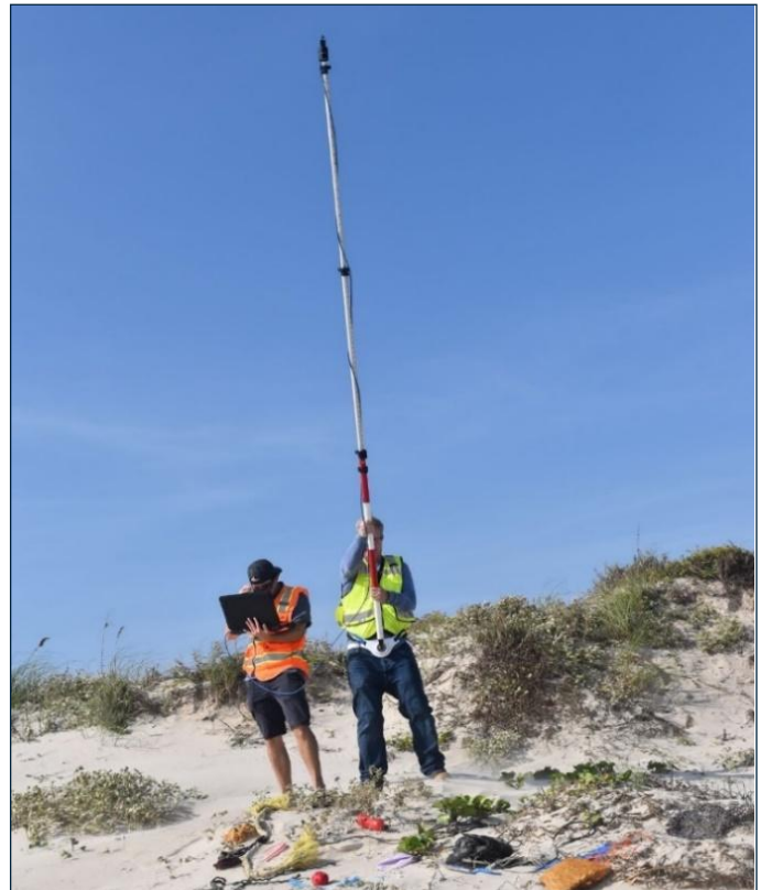
Figure 8: Pole-mounted PI camera collecting imagery of debris on the Texas barrier islands. Credit: NOAA NCCOS.
