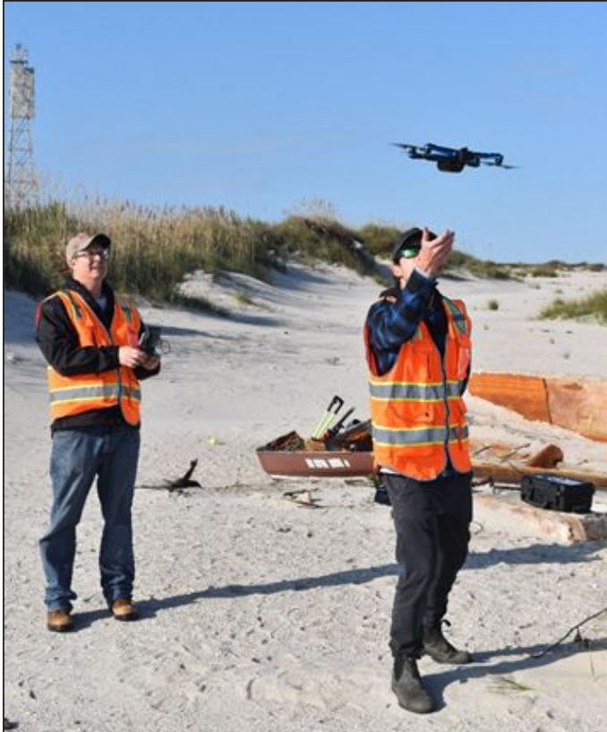
Figure 17: Hand launch of UAS. The aircraft shown here is a Skydio 2. Credit: NOAA NCCOS.
