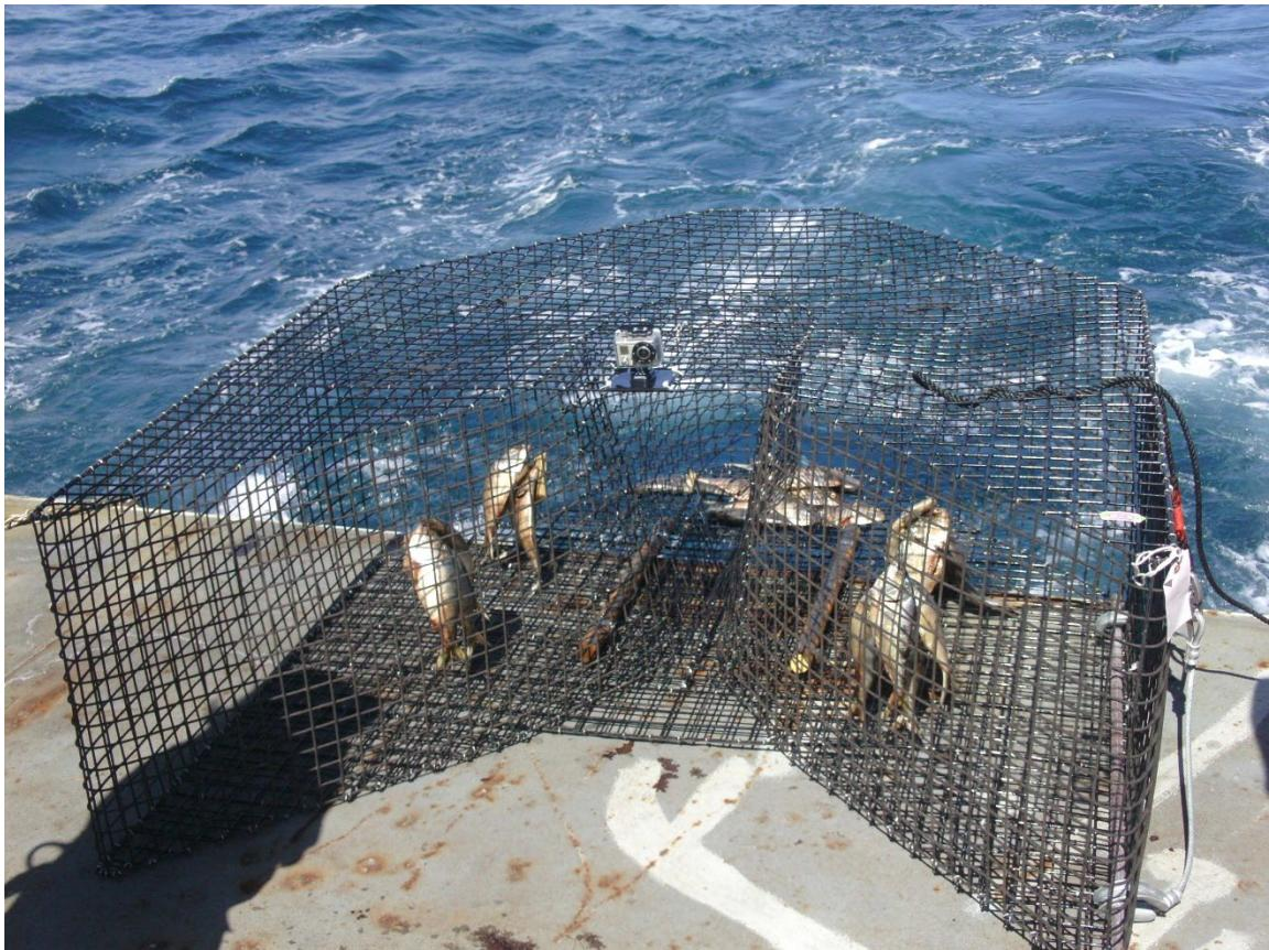
Figure 1. Chevron trap with video camera attached over the mouth position.
