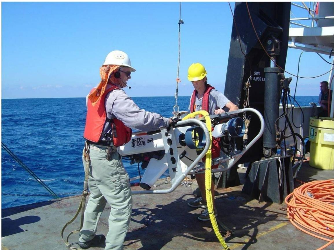
Figure 2. ROV (Super Phantom S2) used on continental shelf and shelf break habitats during leg 2.
