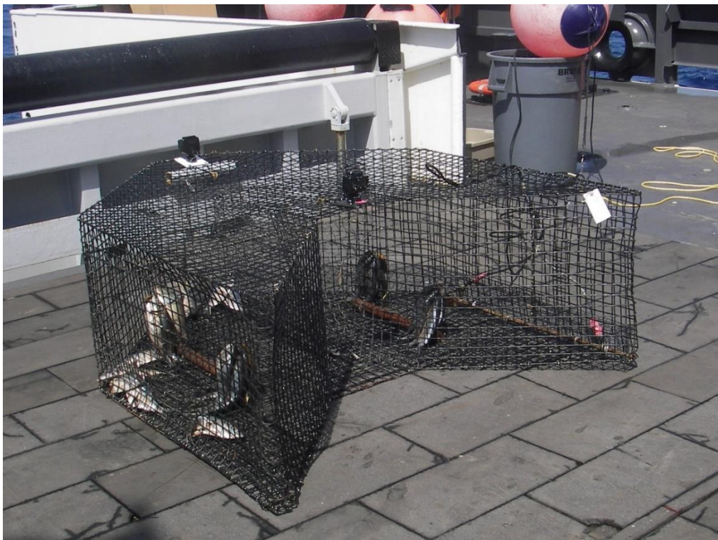
Figure 1. Chevron trap with video cameras used to sample reef fish on the PC-22-03 survey.
