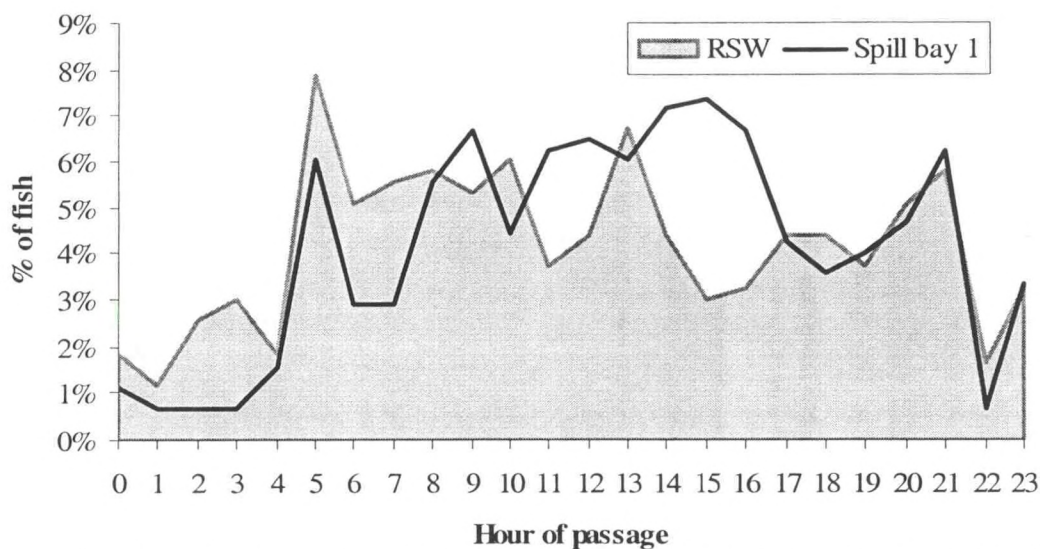
Figure 18. Hour of passage through the Removable Spillway Weir (RSW) and spill bay 1 during RSW spill treatments for radio-tagged yearling Chinook salmon at Ice Harbor Dam, 2005.
