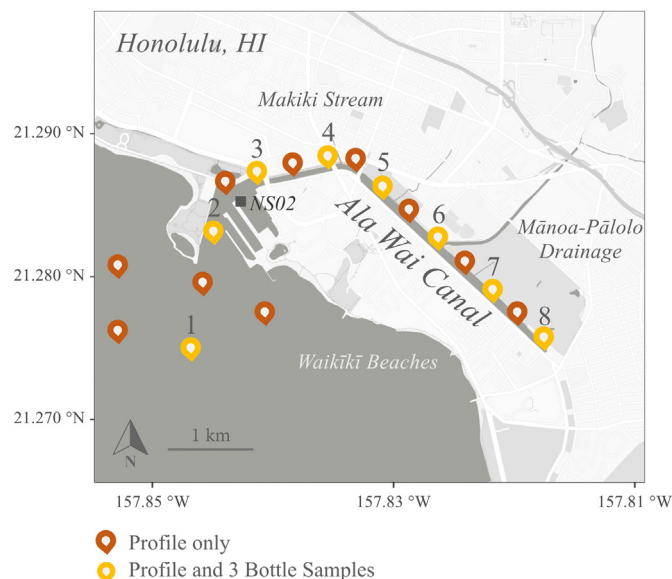
Fig. 1. Map of the Ala Wai Canal in Honolulu, Hawai'i depicting monthly survey sampling locations from October 2018–September 2019. Full depth profiles for salinity, temperature, dissolved oxygen, turbidity, and chlorophyll were collected from all sites ( n = 18 ) marked with a pin. Numbered sites (1–8) are locations where discrete bottle samples were collected at 3 depths (surface, pycnocline, and bottom water) for additional nutrient, organic matter, and microbial measurements. The PacIOOS nearshore sensor NS02 at the Ala Wai Harbor is marked with a grey box.
