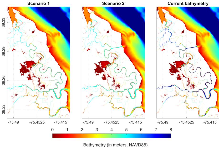
**FIGURE 8** Different channel bathymetry conditions (in meters, from NAVD88 vertical reference level). Left subplot: Scenario 1 - No Sluice Ditch and channel depth 5 m, Mid subplot: Scenario 2 - with Sluice Ditch and depth 5 m, Right subplot: Current bathymetry.
