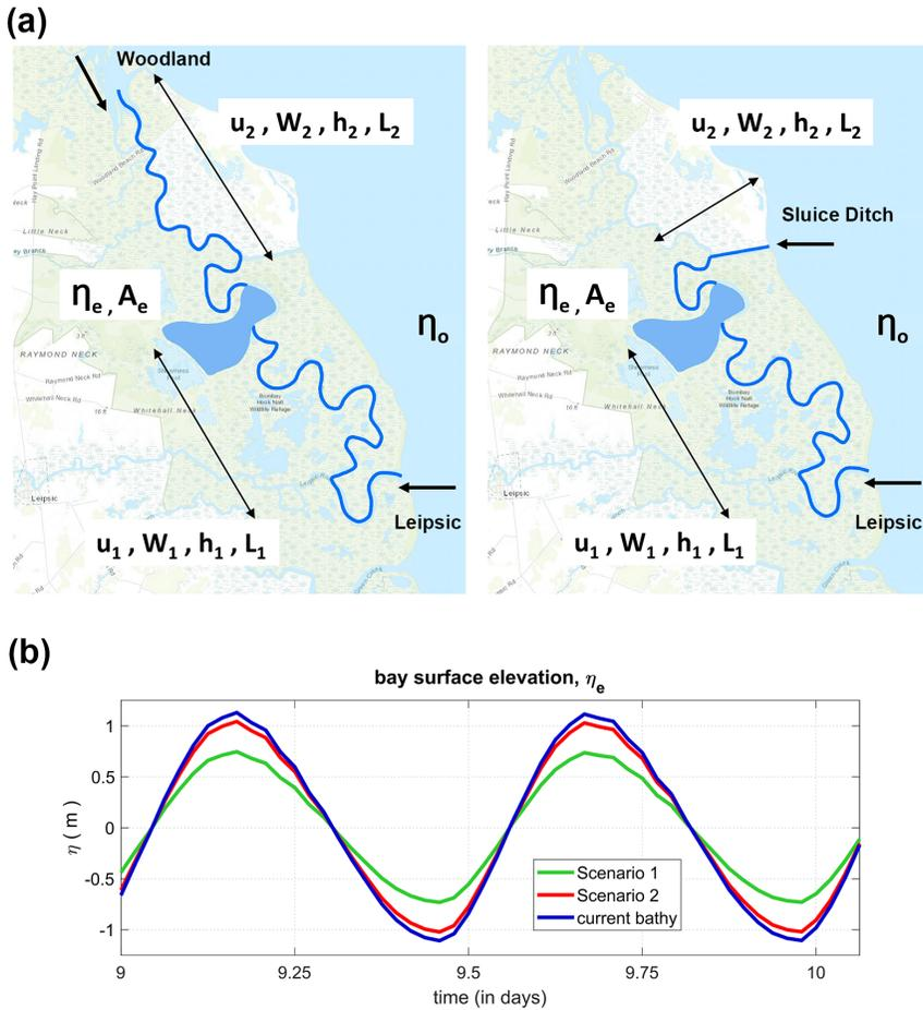
**FIGURE 15** (a) Diagram of the ocean-inlet-bay system inside BHNWR; left subplot: Scenario 1 - No Sluice Ditch, and the interior is connected via Leipsic River and the Woodland beach inlet; right subplot: Scenario 2 and current bathymetry - after introducing Sluice Ditch; (b) Surface elevation,  $\eta_e$  for different morphology scenarios at the Money Marsh mudflat using the analytical model (in meters, from NAVD88 vertical reference level).
