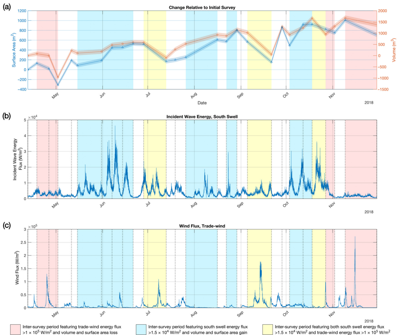
Figure 5. Surface area and volume of the subaerial beach above MHHW (a) plotted alongside incident wave energy flux for south swell (b); wave periods: 14–30 s; wave direction: 147–220°N) and wind flux for trade winds (c); wave periods: 3–10 s; wave direction: 45–160°N). A gradual increase in area and volume throughout the time series: the beach gained 708.5 \pm 43.5 \text{ m}^2 (area) and 1384.8 \pm 102.2 \text{ m}^3 (volume). The overall trend of accretion was interrupted by short-lived erosion events, following which the overall accretion continued. Losses in area and volume coincide with increases in trade-wind energy flux above a threshold of approximately 1 \times 10^5 \text{ W}/\text{m}^2 . Gains in area and volume coincide with south swell energy flux above a threshold of approximately 1.5 \times 10^4 \text{ W}/\text{m}^2 .
