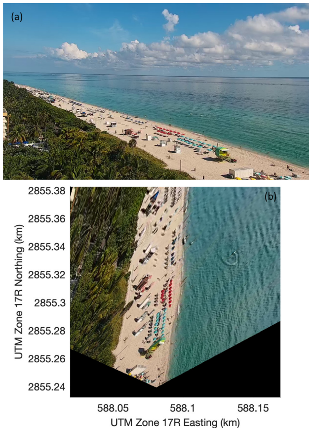
Fig. 3. (a) The calibration image from the WebCAT camera. (b) The rectified planimetric map of the image created using the SurfRCaT-derived calibration.
