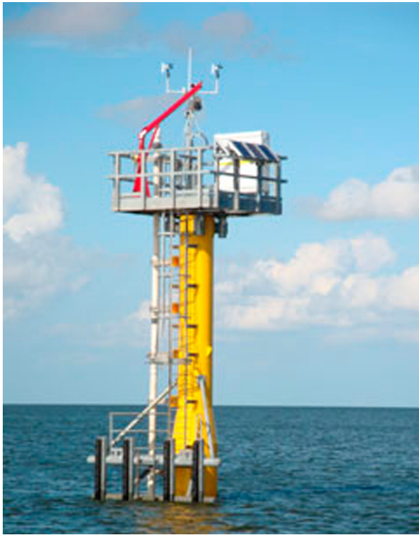
Figure 2. 'NOAA Sentinels' are water level stations designed to withstand wind and wave action from category four hurricanes (winds from 131 to 155 miles per hour).
