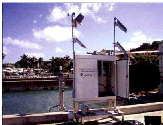
Figure 17. Tsunami tide station in Christiansted, Virgin Islands.
