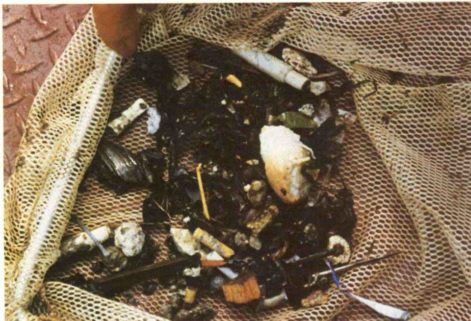
Screened materials collected from effluent plume. (Passaic Valley Sewerage Commissioners' Plant. (See sec. 4.3.)
