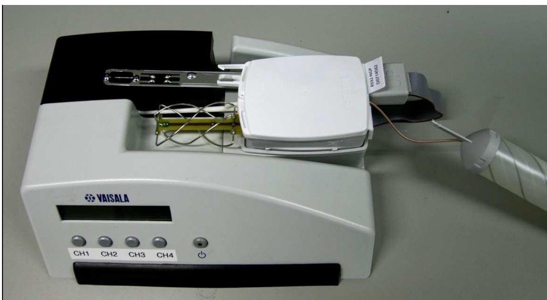
Exhibit F-6 Correct placement of the radiosonde in the Frequency Setting Device
