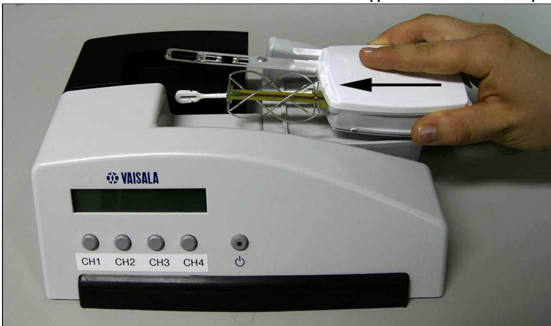
Exhibit F-5 Placing the radiosonde in the Frequency Setting Device
