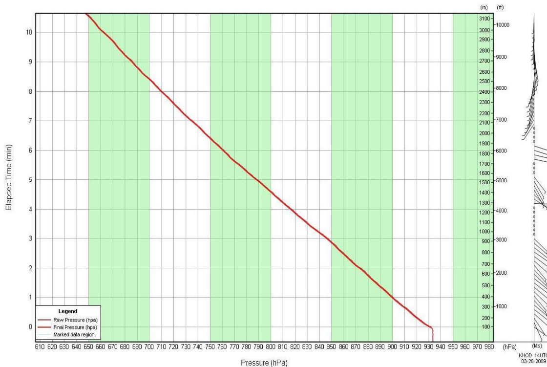
Exhibit 5-21: Pressure data plot for the first 10 minutes of the sounding
