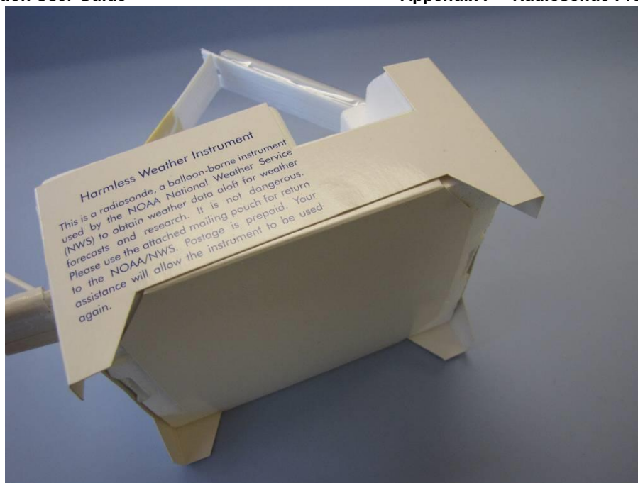
Figure 7 - Sealing the bottom of the sleeve.
