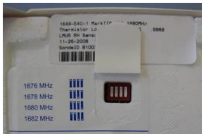
Figure 3 – Changing the Dipswitch
