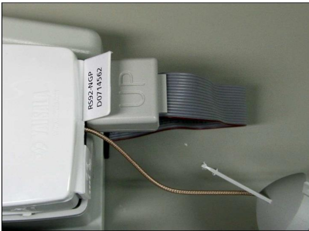
Exhibit F-7 Connecting the communication cable
