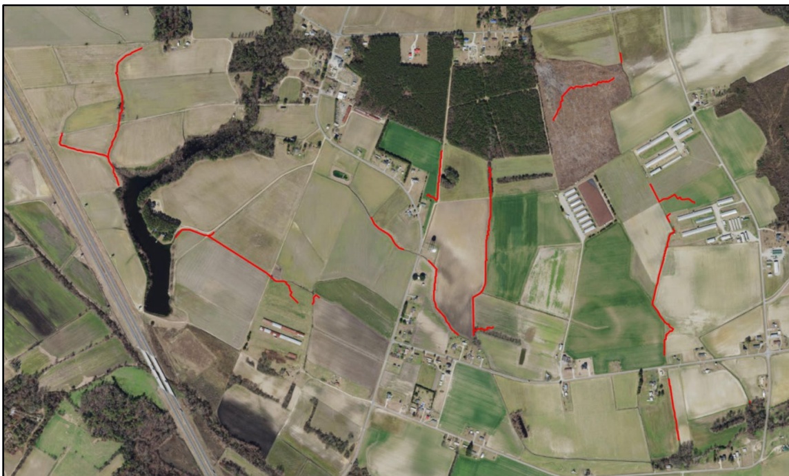
Figure 4-6. First and second order channels on agricultural land after removing floodplain areas and buildings.
