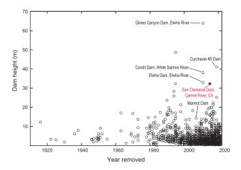
**FIGURE 1** Dams removed intentionally in the United States, 1912 to 2021 (data from American Rivers, 2021). These include 1785 dams (shown on plot) and another 144 with unknown removal date. Names of the largest dams discussed in the text are indicated: San Clemente Dam, Carmel River, California; Elwha and Glines Canyon Dam, Elwha River, Washington; Cucharas #5 Dam, Colorado; and Condit Dam, White Salmon River, Washington.
