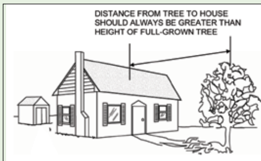
Figure 5-24. FEMA recommends that the distance between a tree and your house should always be greater than the height of the full-grown tree. This is to prevent trees from falling on the roof, either currently or in the future. Image courtesy of FEMA
